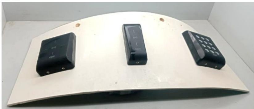
**Purpose of Test:** To check the resistance of materials and surface coatings of a system/component against salt mist
