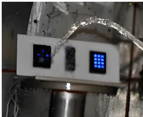
**Purpose of Test:** Equipment Under Test (EUT). Protected against low-pressure jets of water from any direction – limited ingress permitted
