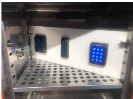
**Note:** The readers were tested under temperature of -40°C but the recommended operating temperature is -30°C.
