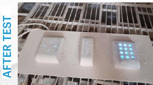
**Purpose of Test:** To evaluate the ability of the device to resist the effects of dust
